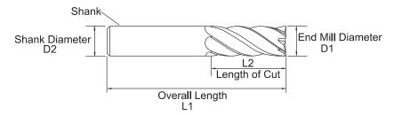
Length of Cut (Flute Length) – Always select the shortest Flute Length possible for your application. By selecting the shortest Flute Length, you can increase rigidity and allow for higher feed rates.
